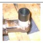
4. Remove the Grout Port out of the tool and press by hand without turning into the drill hole up to the marking. Keep it fixed by hand and push spread tool through the grout port hole in full depth and hold on with low pressure for 10 seconds for perfect fixing. Fixing is finalized
