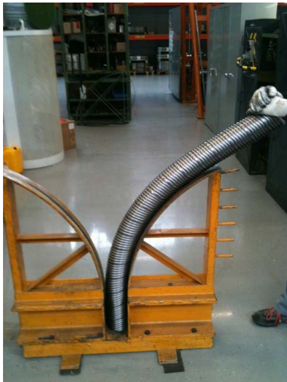
PT 1 C2 Steel duct flex behaviour test acc. 524-2
