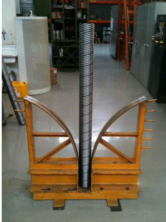
PT 1 C2 Steel duct flex behaviour test acc. EN 524-2
