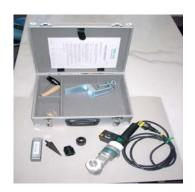
The welding equipment consists of 2 parts (welding machine and drill tool). You might use a block of wood for intermediate storage of heated welding equipment.
