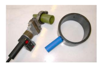
This general Plug Welding operation manual is provided to weld all kind of plugs into smooth pipes e.g. closing plugs, anti-noise distance plugs, exit plugs and pipe plugs. The welding equipment consists of 3 parts (welding machine, drill tool and deburring tool. In addition you might use a wood block for intermediate storage of heated welding equipment.
