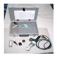
The welding equipment consists of 2 parts (welding machine and drill tool). You might use a block of wood for intermediate storage of heated welding equipment. The plugs can be used for corrugated PES.TEC pipes IP-1, PES.TEC pipes IP-2 and IP-3, PT Plugs, GTI and others and all kind of smooth ducts.
