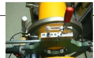
20. After minimum circumferential adjusting bead is achieved, release the pressure to the warm up pressure indicated in the list.
