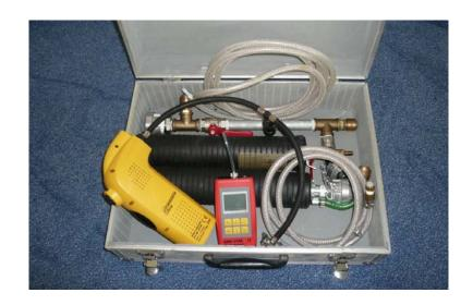
The Leak Tightness Test Equipment suitable for pipe ID 70 – 150 mm (3-5 inch) for max 0.25 bar (3,5 PSI) consists of following parts
